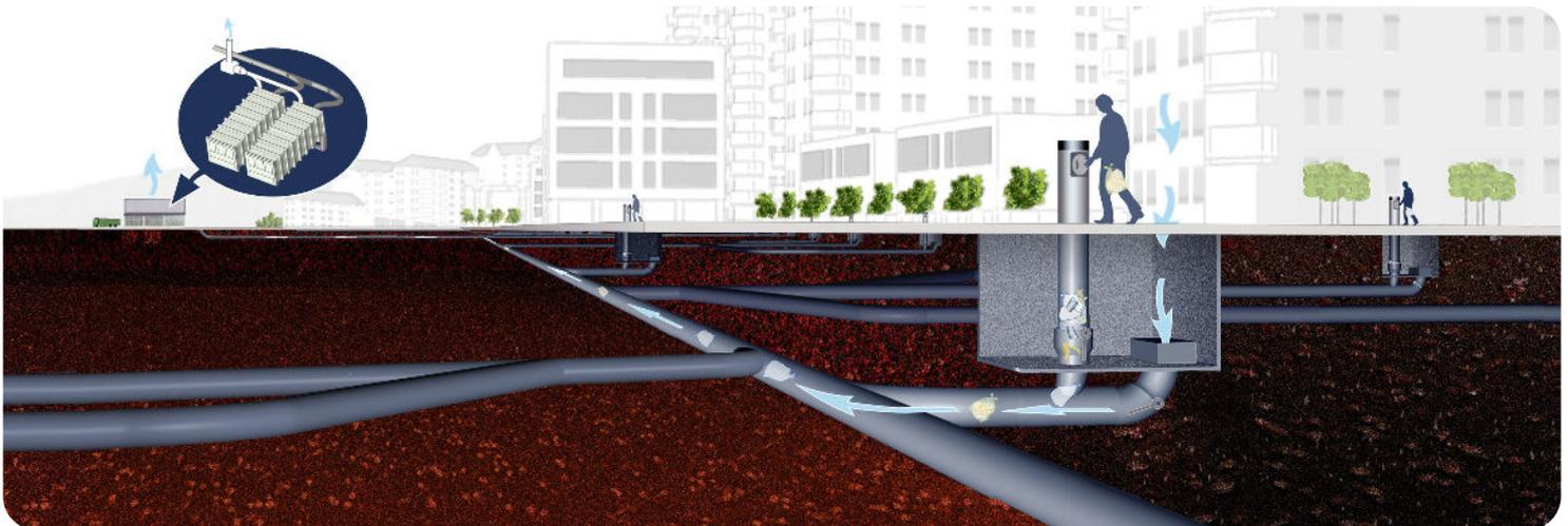
A vacuum waste system is collecting the residual waste in your area. The only thing you can see of the system is the inlets. The picture above shows how a vacuum waste system works.
